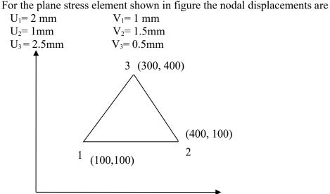
Determine the element stresses. Assume E=200GN/m<sup>2</sup>,  $\upsilon = 0.3$ , t= 10mm. Use Gaussian Quadrature to obtain the exact value for the following integral. 6 [14M]  $\int_{-1}^{1} (r^3 - 1)(s^2 + s) dr ds$
