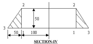
7 A composite wall consists of three materials, as shown in Fig. The outer [14M] temperature is To = 20°C. Convection heat transfer takes place on the inner surface of the wall with T $\alpha$  = 800°C and h = 25 W/m<sup>2.o</sup>C Determine the temperature distribution in the wall.
