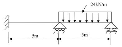
8 Determine the Eigen values and Eigen vectors for the beam shown in figure
